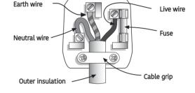
The wire coloured **BROWN** is the **LIVE** wire and must be connected to the terminal marked L or coloured **RED**.
