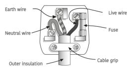
The wire coloured **BLUE** is the **NEUTRAL** and must be connected to the terminal marked N or coloured **BLACK**.
